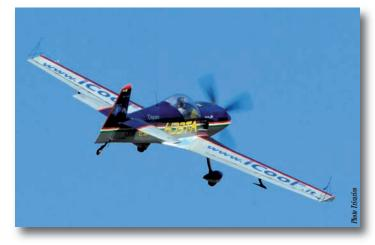
Its structure is entirely wooden with Okoume-, 2mm plywood skin and a reinforcement layer in bifilar-, 45° fiberglass added later to increase strength and withstand load factor up to +/-10g.
